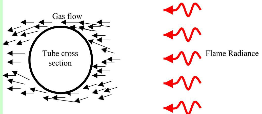
In the simple drawing above we illustrate convective gas flow, which is turbulent, and radiant heat from the flame, refractory and other tubes – all non-uniform and time varying. When you view tube from an access port typically you can only see a portion of the tube or the tube at an oblique angle. Therefore, the odds are stacked against you from the start!
