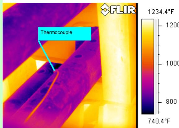
The emissivity of the tube surface is very tough to determine and typically is derived from two sources – correlated to thermocouple measurements or folklore (“we’ve always assumed 0.88”). The former process is tough to accomplish but the preferred method. The latter has value in that existing trend data may exist. We are working on a better method of measuring process heater tube emissivity and will report on it in the future!
